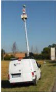
Level-Lift Roof Evo is conceived in order to take advantage to the Level-Plane EVO for land surveying, infrastructures, architectural and structural reliefs. It's composed of 4 pneumatic extensible segment (max 3.00 m height), a support plate for Level-Plane EVO and a frame that allows the mounting on the vehicle roof rack. The solid structure of the aluminum frame, holding the pole and its components. It's adaptable to any vehicle.
