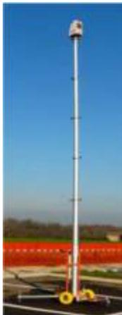
Kangur-Lift is a telescopic column made of anodized aluminum with pneumatic extensions by hand pump, complete with manual locks that allows to stop the column at the desired height, with maximum height of 6.00 meters. The column is mounted on a cart with rubber wheels and painted frame, with light and compact design. Provided with adjustable feet combined with a spherical bubble to ensure the vertical position of the pole and a set of windbracing ropes.
